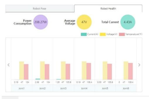
**Note** The monitoring values are displayed when the robot is running normally.
