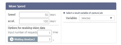
You can set the movement speed/acceleration for a vision camera attached in the robot to move to the recording location.
