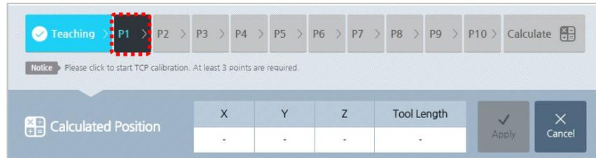
4. While pressing down the **Direct Teaching** button in the **Manual Move** screen, move the robot arm to place the tip of the tool right at the reference point.
