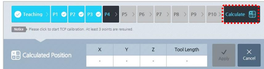
8. Check the calculated position result and press the **Apply** button.
