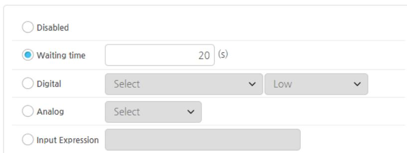
The screenshot shows a configuration panel for the WAIT command. It features five radio button options: Disabled, Waiting time, Digital, Analog, and Input Expression. The 'Waiting time' option is selected, with a text input field containing '20' and a '(s)' unit label. The 'Digital' option has two dropdown menus, one set to 'Select' and the other to 'Low'. The 'Analog' option has a dropdown menu set to 'Select'. The 'Input Expression' option has a large, empty text input field.
